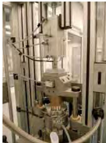
Figure 1. The MSS-2 reactor for solvothermal synthesis of nanoparticles. MW power 3 KW, volume 470 ml, maximum pressure 6 MPa, temperature 260oC.
