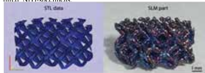
Fig.1: STL data and SLM part of a NiTi lattice structure.
