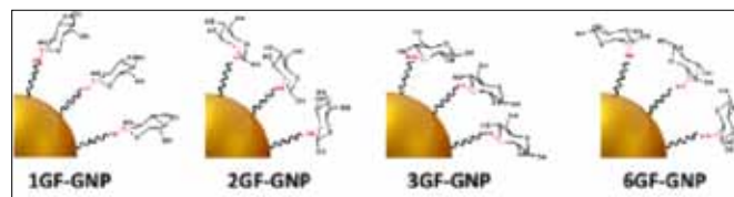
Figure 1: Selective uptake of 2GF- GNPs. A) Schematic diagram of the four distinct GF-GNPs, with the same shape and size, differing only in the intra-molecular glucose conjugation site (C 1 , C 2 , C 3 and C 6 ).
