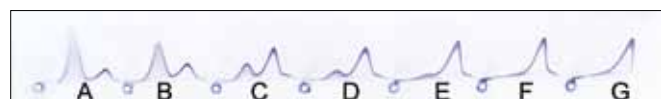
Figure 1: Serie of electrophoregrams obtained for increasing surface of NPs made with Isobutylcyanoacrylate grafted with Dextran 67 kDa, 1.3% 5 .
