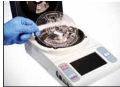
Fig.1. Foil-based disc-shaped microfluidic cartridge (LabDisk) and the corresponding Lab-Disk Player, integrating user-defined frequency and temperature protocols as well as an optical detection unit (fluorescence).
