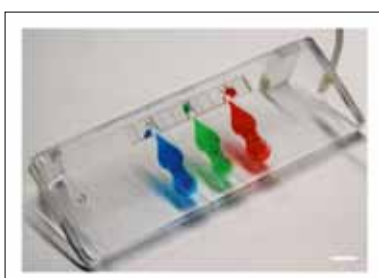
Fig. 1. Lung on chip that mimics the thin alveolar barrier as well as the cyclic mechanical strain induced by the respiration (from (3)). Scale bar: 5mm.
