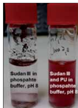
Increased water solubility of sudan III in presence of PU, at pH 8.
