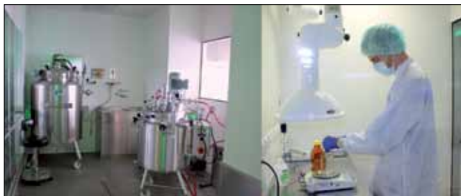
Figure 1: Facility of the Pharmacy Department, Erlangen University Hospital for the production of iron oxide nanoparticles in a scaled up manner under GMP conditions.
