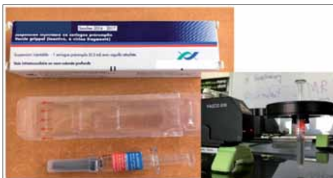
Figure 1: The commercial vaccine syringe out of its blister (left); Measurement setup principe (right) with the remote head mounted on a dedicated translatable stage and placed in front of a syringe holder designed for the purpose of the experiment (see insert)
