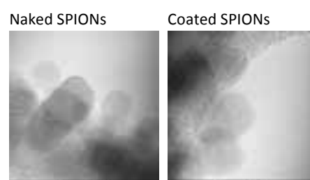
Fig. 1: High-resolution transmission electron microscopy micrographs showing the iron oxide surface of naked SPIONs versus
