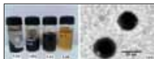
Fig. 1: Uncoated SPIONs (a), Aqueous ferrofluid (b), Curcumin loaded ferrofluid (c) CUR-SPIONS diluted with water (d), TEM image (e).
