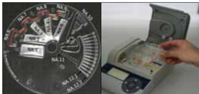
Fig.1: The LabDisk and Reader. The sample (50µl whole blood inserted in NA.6) is treated with buffers (pre-stored on disc in pouches called "stickpacks" in NA.1-NA.5) for pathogen lysis, DNA/RNA extraction (presence of magnetic beads) and purification. The purified (eluted) nucleic acid is pumped from NA.9 to NA.11 where it rehydrates a lyopellet, which contains amplification enzymes, dNTPs. The mixture is then aliquoted (via the microfluidic module NA.12.1) to the reaction chambers (NA.12.2) where the pre-stored primers initiate the LAMP amplification, which is detected in real time via fluorescence.
